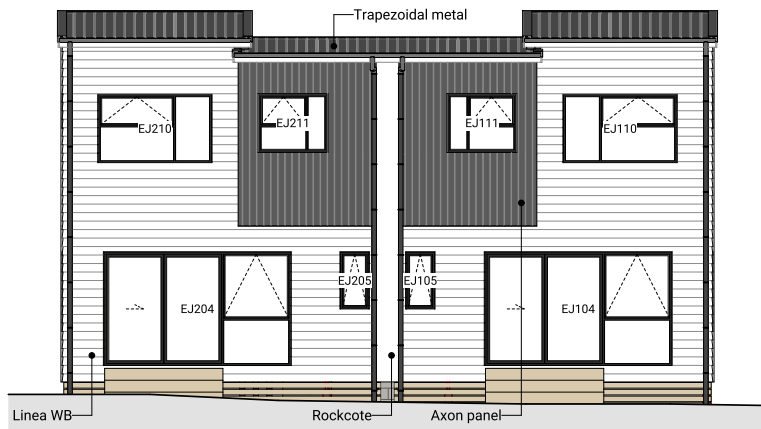
3 North West Elevation
